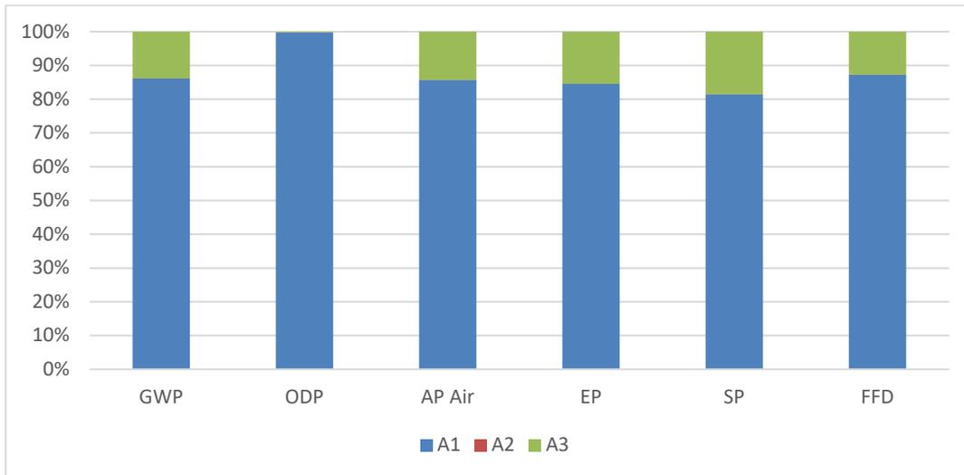
Figure 4 - Relative Contributions of Cradle to Gate Life Cycle Stages for Wet Coated Glass
