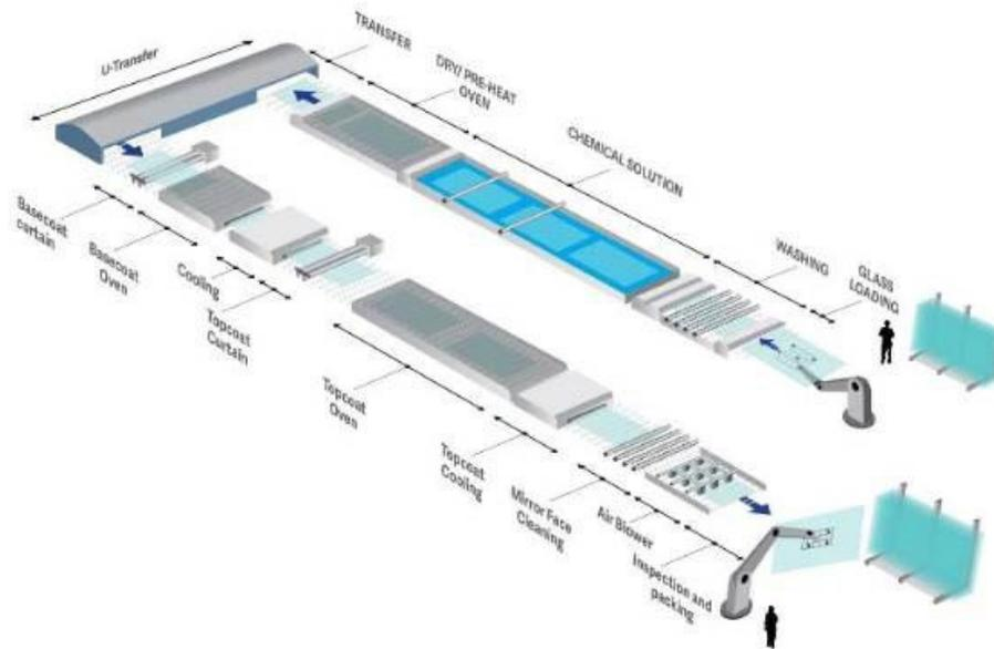
Figure 3 – Wet Coating Mirror Production Process
